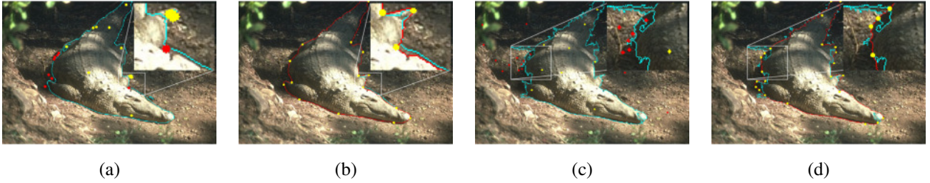
Figure 7: Crocodile image segmented with (a) fBRS (cyan contour) from internal (yellow) and external (red) clicks. Grabber provides (b) higher boundary adherence with less effort (red contour, previous contour in cyan). (c) Segmentation with DT from object (yellow) and background (red) markers. (d) Correction with Grabber (red contour, previous contour in cyan).
