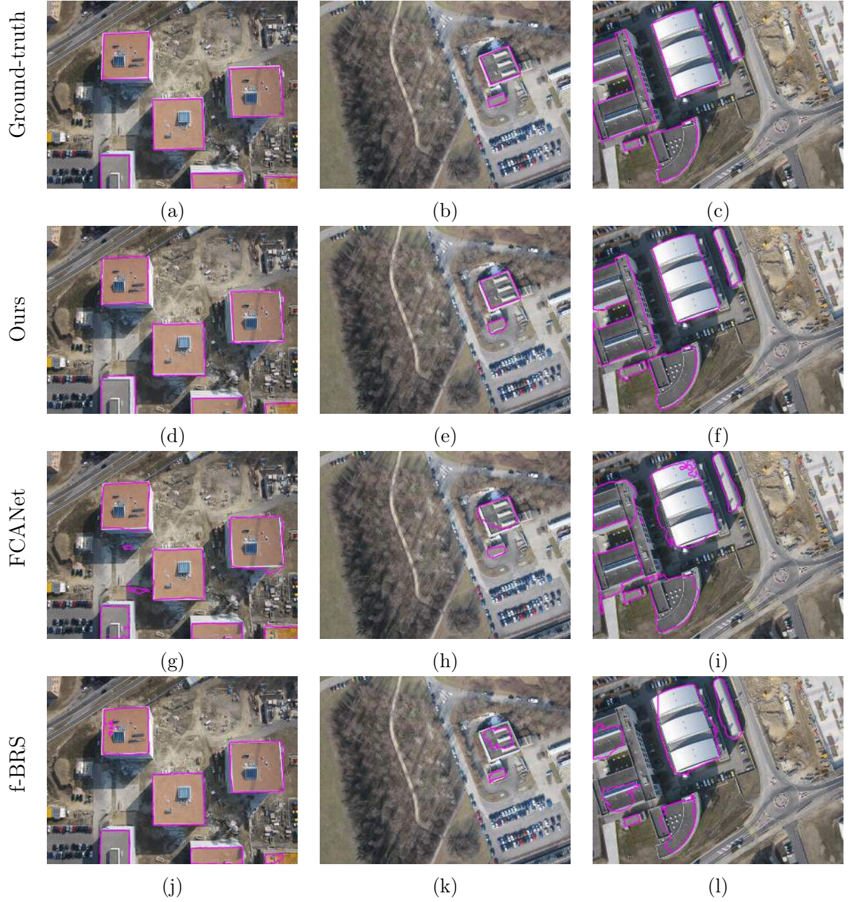
Figure 5.8: The magenta boundaries delineate regions with foreground labels for the ground-truth data, our method, and the baselines using 5 clicks per instance on the Rooftop dataset.
